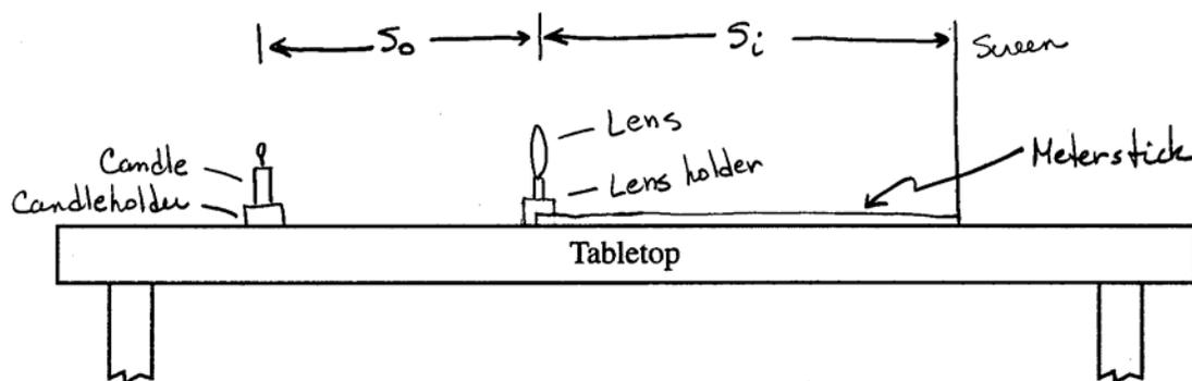
For showing a functional setup involving an object, the lens, and a screen
