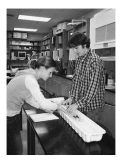
Students use an inexpensive wallpaper tray as a water bath for the cell respiration lab (AP Lab 5). When doing this lab with your students, be sure to allow the vials a full 15 minutes to stabilize. Use a thermometer in the tray to record possible temperature changes. (Photograph courtesy of Carol Leibl.)
